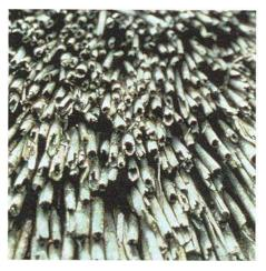
Fig 24 Water reed (Photograph copyright @ John B Letts)
